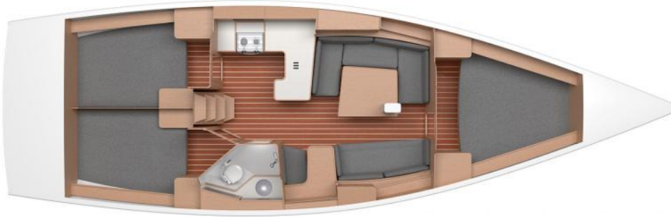
Arcona 415 interior layout - 3 cabin, single WC - standard
