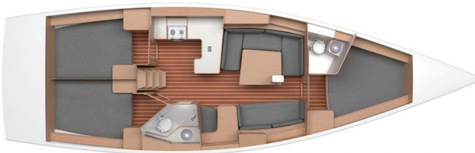
Arcona 415 interior layout - 3 cabin, double WC - upgrade option
