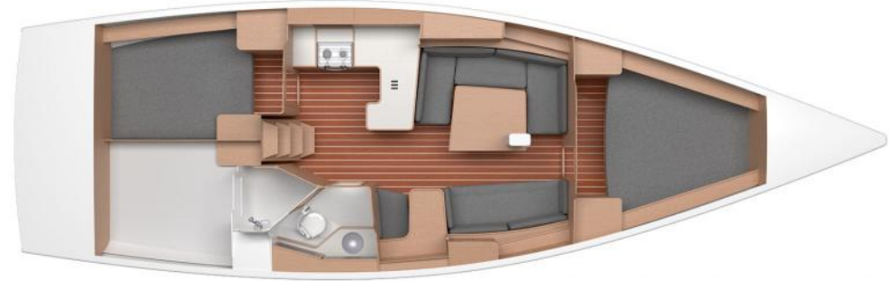
Arcona 415 interior layout - 2 cabin, single WC, with large shower - upgrade option
